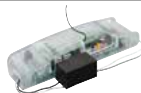
For controlling the LED strips LT ES 11 to LT ES 61.
